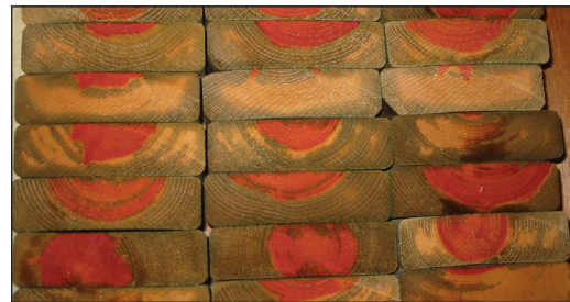
Figure 2. Example of preservative distribution in 2 by 6 lumber (nominal). The brown color is the preservative and the red color is heartwood.
