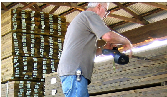
Figure 1. The retention in a charge of treated lumber is determined by removing increment cores from 20 pieces and combining them for a single assay value.
