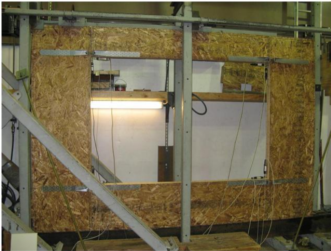
Figure 4—Wall 5, with intermediate length load head; note the instrumented hold-downs which were used in lieu of flat straps.
