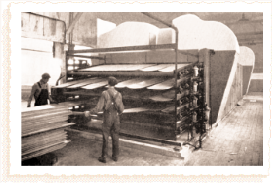
Wet and dry ends of a Coe Model 28 veneer dryer at Robinson Manufacturing Company, Everett, Wash.
