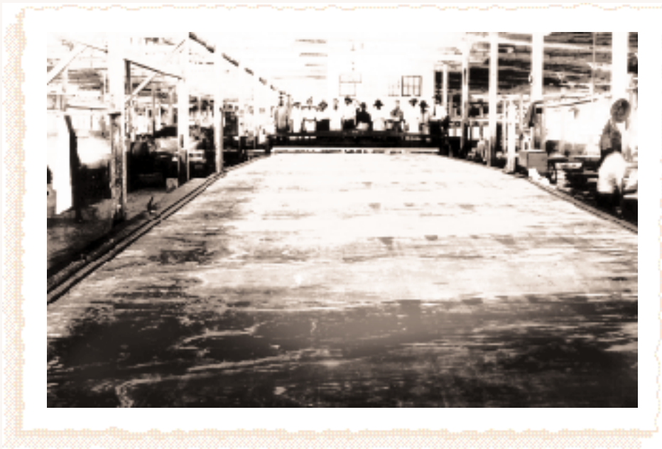
This 1920 era picture shows a 60 ft.-by-16 ft.-8 in. veneer sheet from "the world's largest lathe" - Coe's installation at Flora American Plywood Company in Macon, Georgia.
