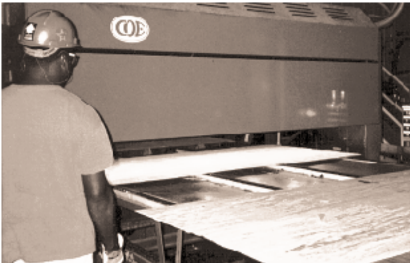
The Coe Veneer Grade Scan system for automatic sorting and stacking in plywood mills is typical of the leading edge technology flowing from the company's ongoing research and development efforts. The recently-introduced scan system makes accurate grading decisions piece by piece. Defects are extracted with the help of high-speed image processing computers. Software evaluates the optimum grade based on entered grading rules.
