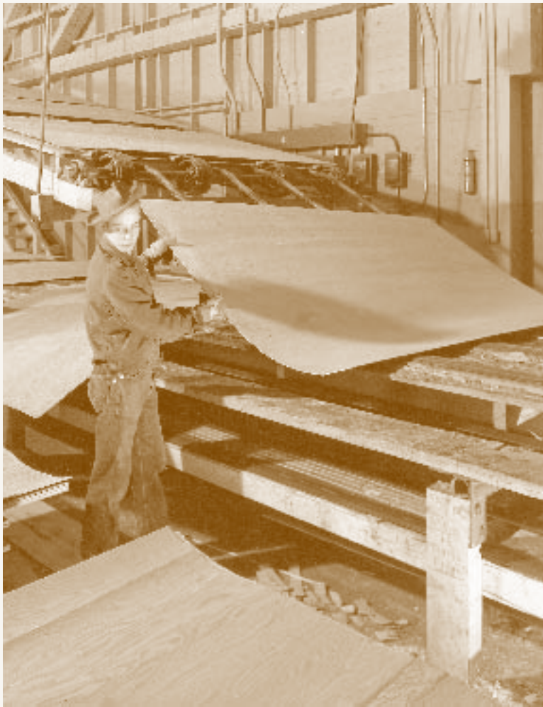
Pulling veneer off the green chain
