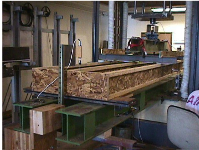
Figure 1. Test setup for bare I-joist frames
