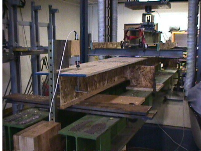
Figure 3. Test setup for T-beam assemblies
