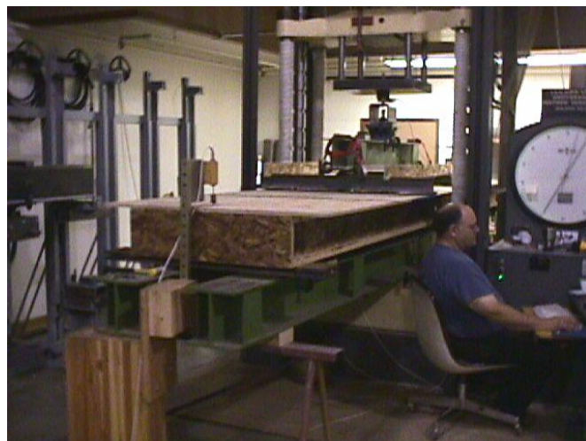
Figure 2. Test setup for I-joist floor assemblies
