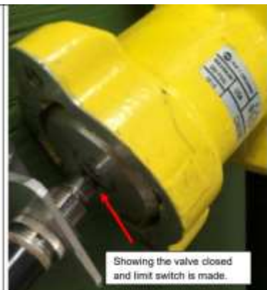
Photo of the valve modification. When the valve is closed it threads through the plywood making the limit switch located on the back.
