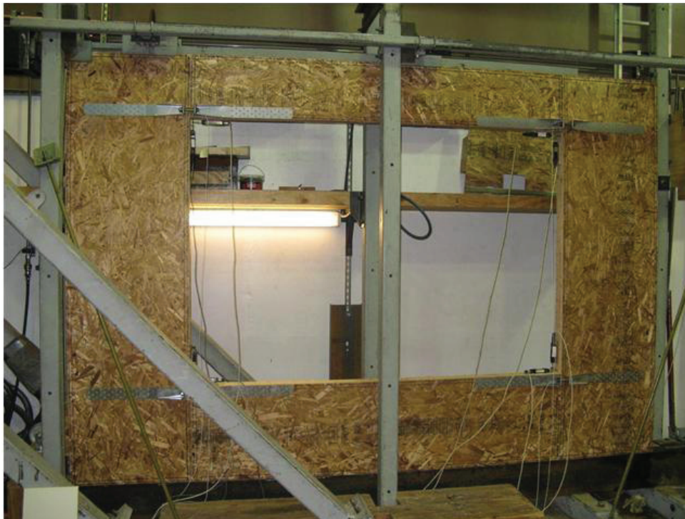
WALL 5A, WITH “INTERMEDIATE” LOAD HEAD (PAINTED GRAY)
