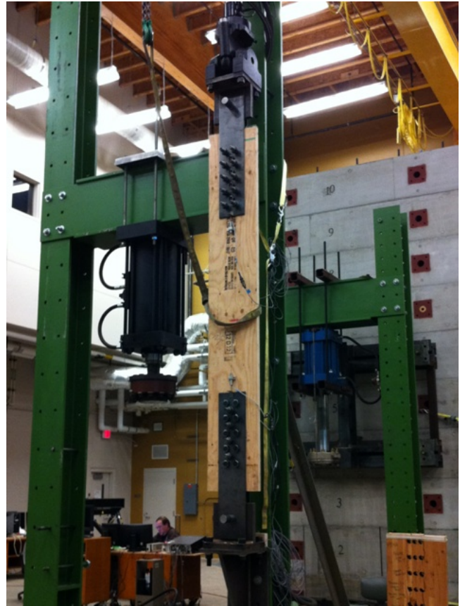
Figure 3: Multiple bolted connection test setup
