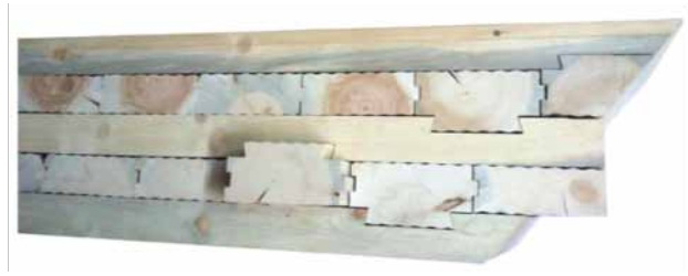
Figure 1. Cross section of an ICLT panel showing tongue-and-groove joinery and dovetail joinery. Photo by Ryan Smith
