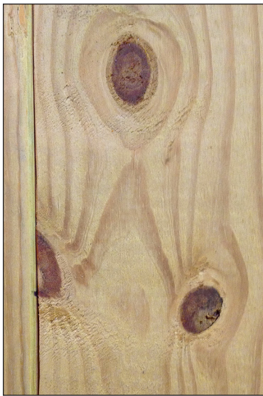
Figure 1. Multiple knots in close proximity found in southern yellow pine lumber.
