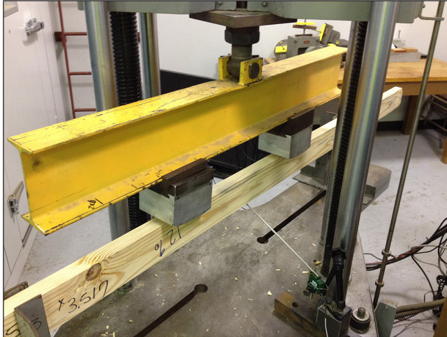
Figure 2. Mechanical testing of specimens in an Instron universal testing machine.
