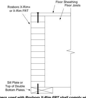
Fasteners used with Rosboro X-Rim FRT shall comply with the recommendation provided by the FRT treater
