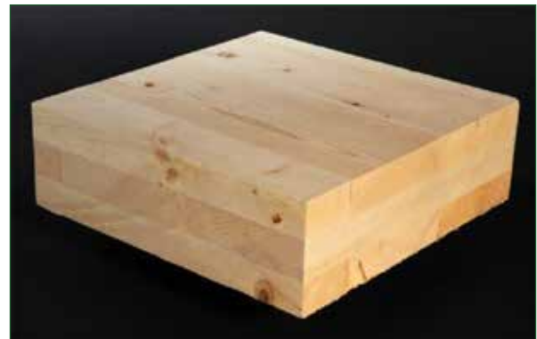
Example of CLT panel with three layers.
