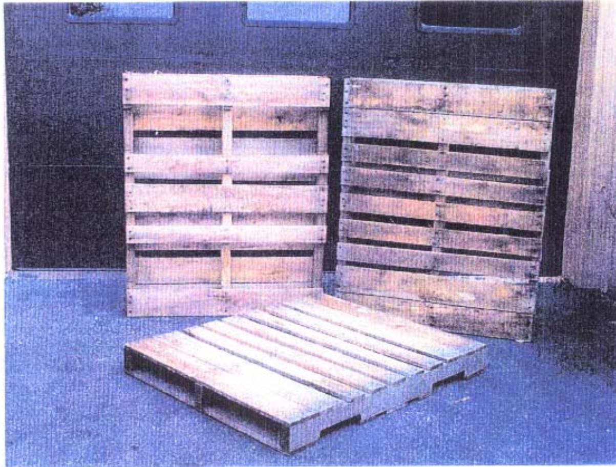
Figure 3. A photograph of the lumber/stringer pallets tested.
