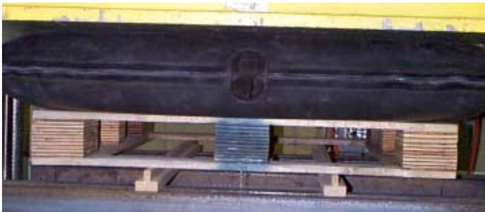
Figure 7: A photograph and schematic view of the conveyor simulation tests with the supports placed parallel to the pallet length.
