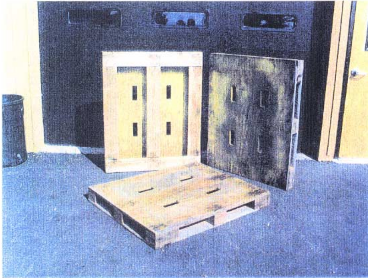
Figure 1. A photograph of the full panel deck pallets tested.
