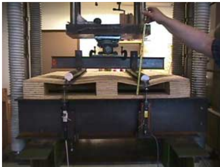
Figure 7. Top deck bending failure in top deck bending test
