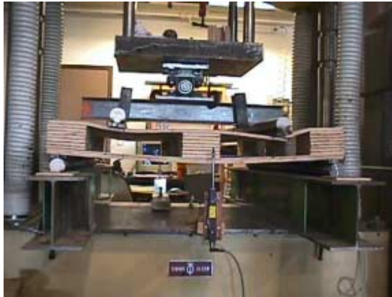
Figure 6. Top deck bending failure in racking test
