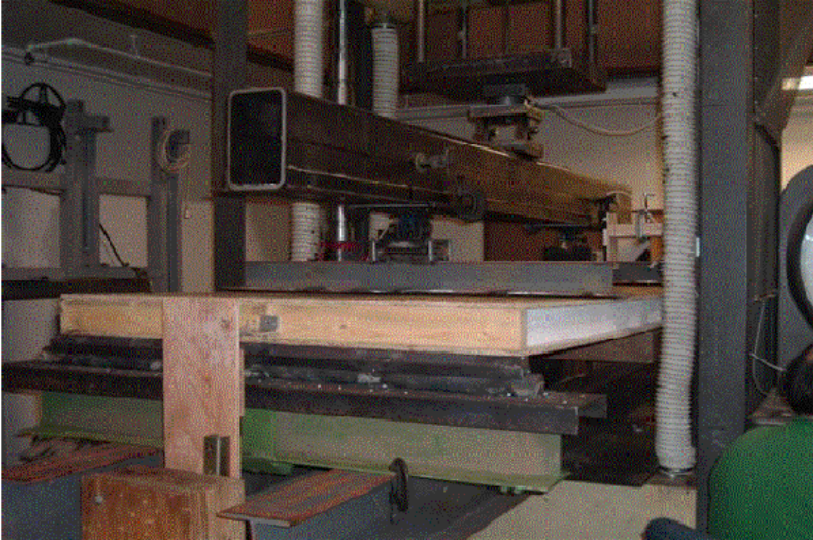
FIGURE C1. SIPS PANEL IN TRANSVERSE LOAD TEST APPARATUS – THIRD-POINT LOADING APPARATUS (File Picture)
