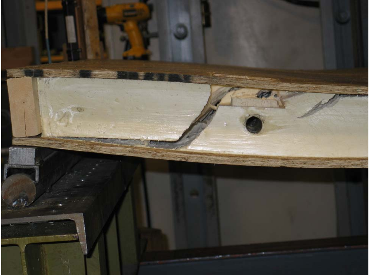
FIGURE C3. TYPICAL SIPS TRANSVERSE LOAD FAILURE (Shear failure of core in vicinity of lower conduit chase)
