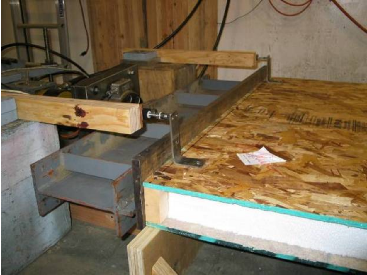
FIGURE B4. AXIAL (COMPRESSION) LOAD TEST ASSEMBLY – LOAD HEAD WITH INSTRUMENTATION
