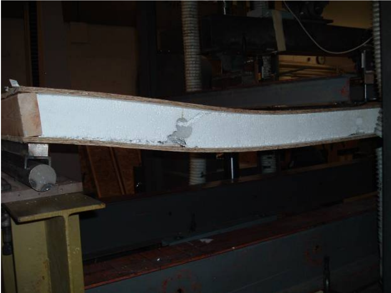
FIGURE C5. TRANSVERSE LOAD TEST (Fully propagated failure on tension side at electrical chase holes - typical)
