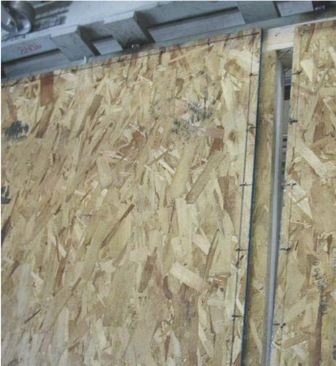
FIGURE C1. RACKING SHEAR TEST FAILURE (Nails tear away from center spline)
