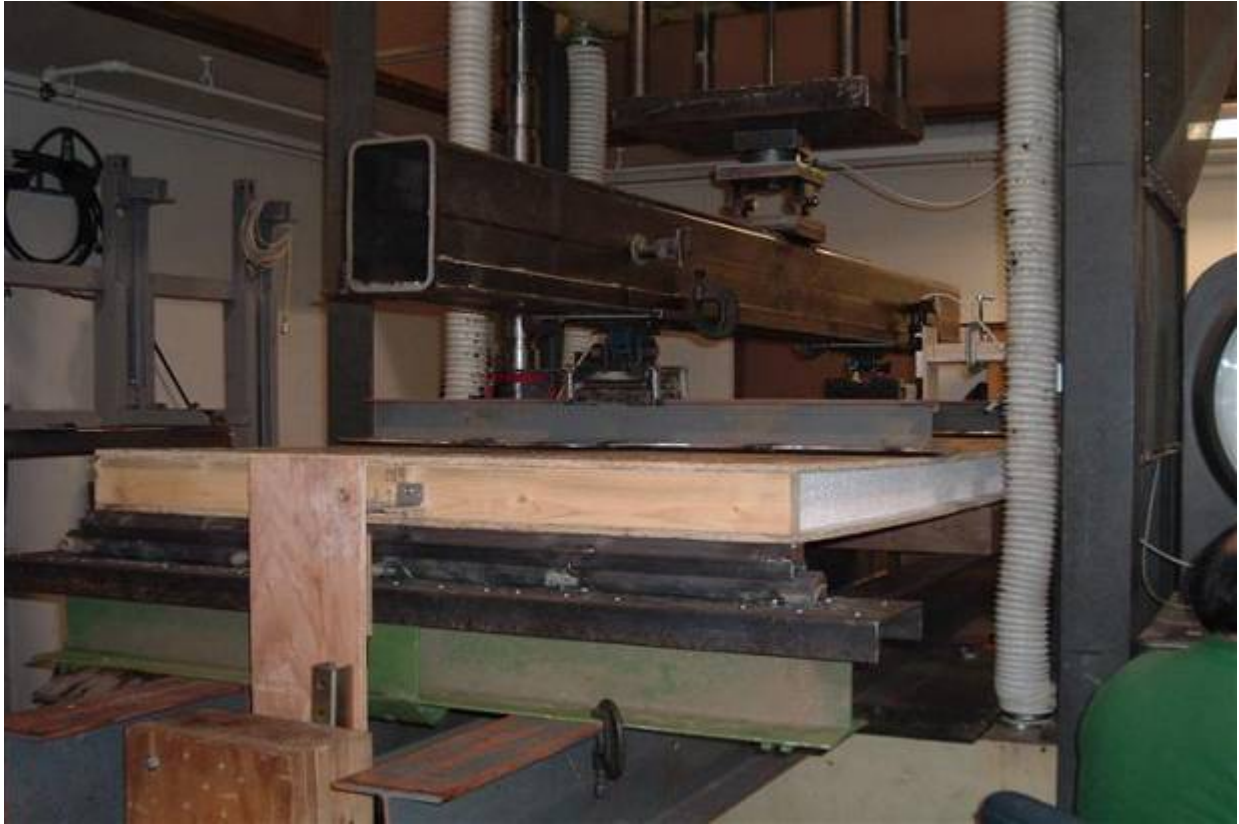
FIGURE B7. TRANSVERSE LOAD TEST ASSEMBLY
