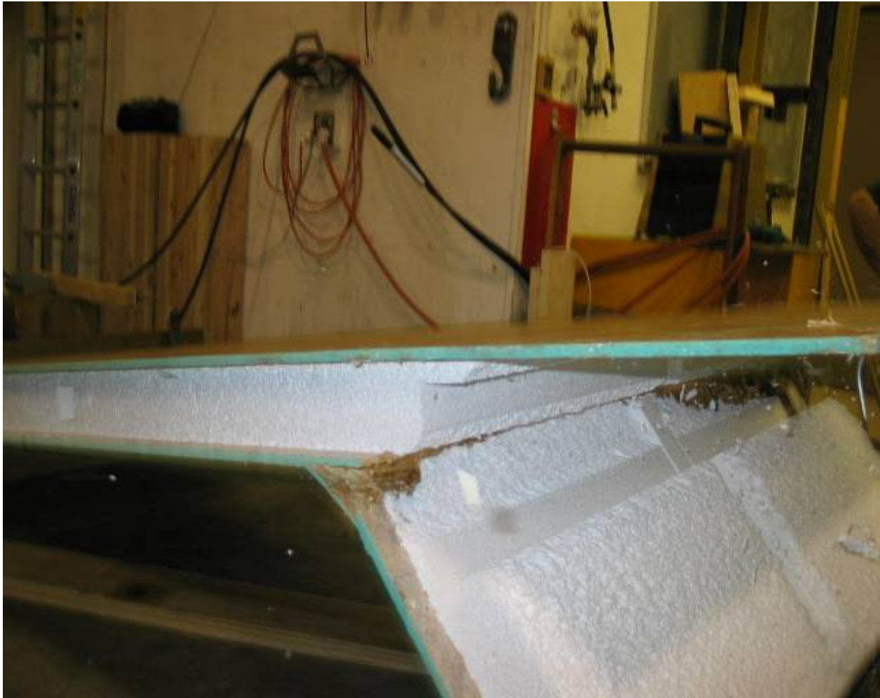
FIGURE C3. AXIAL LOAD (COMPRESSION) TEST (Fully propagated shear failure through foam propagated from horizontal electrical chase at bottom edge of panel - typical)
