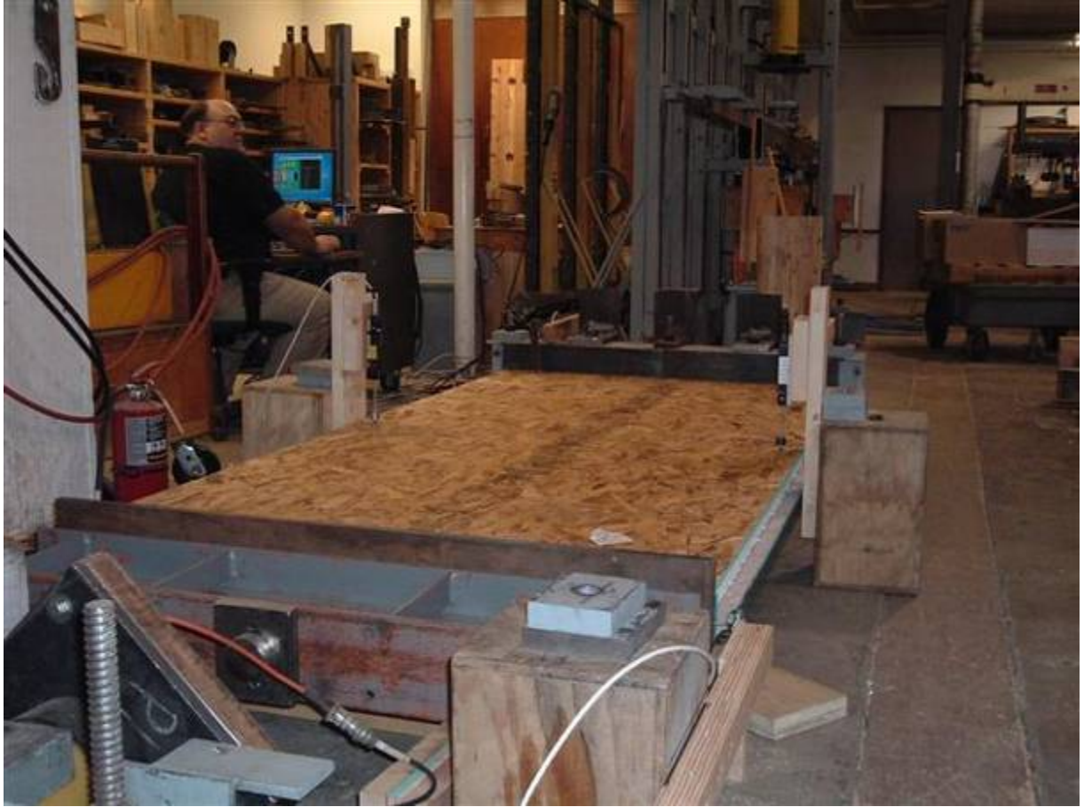
FIGURE B3. AXIAL (COMPRESSION) LOAD TEST ASSEMBLY
