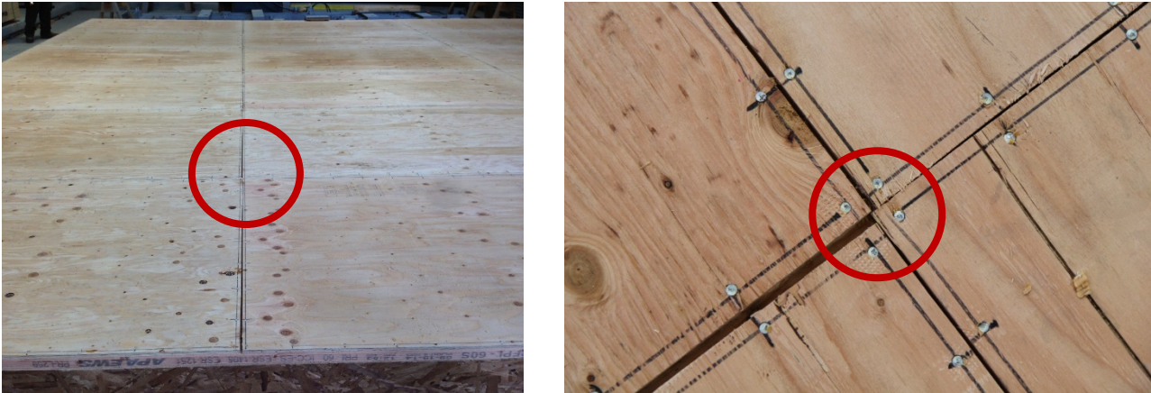
Figure 1. Deformation shape of a light-frame diaphragm showing the corner joint as circled
