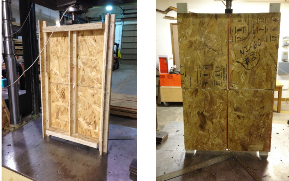
Figure 3. Actual assemblies for small-scale diaphragm tests
