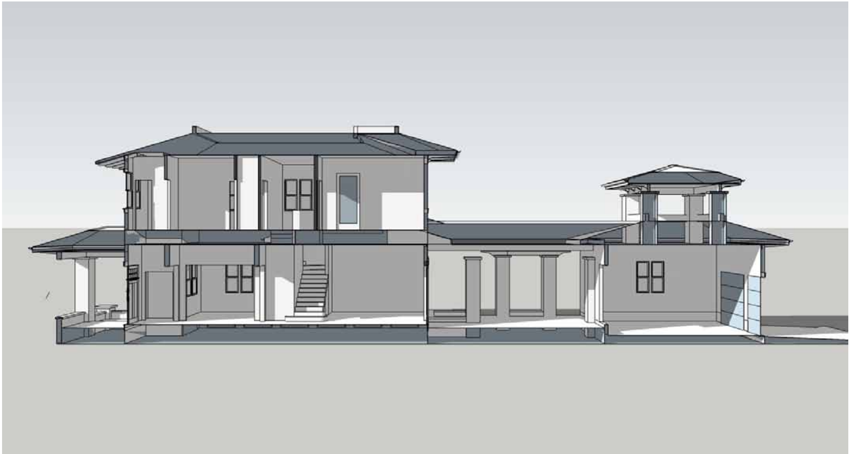
Longitudinal Section Florida Carbon Challenge - Entry No. 135
