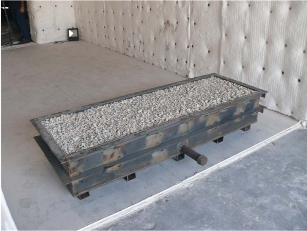
Figure X2-5. Propane Diffusion Burner
