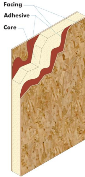
Figure 3. Example of a SIP Wall Panel (adhesive is not required with the polyurethane core)
