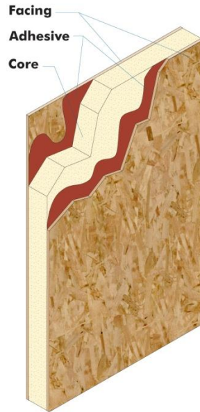
Figure 3. Example of a SIP Wall Panel (for foamed in place foam cores, the foam is the adhesive)
