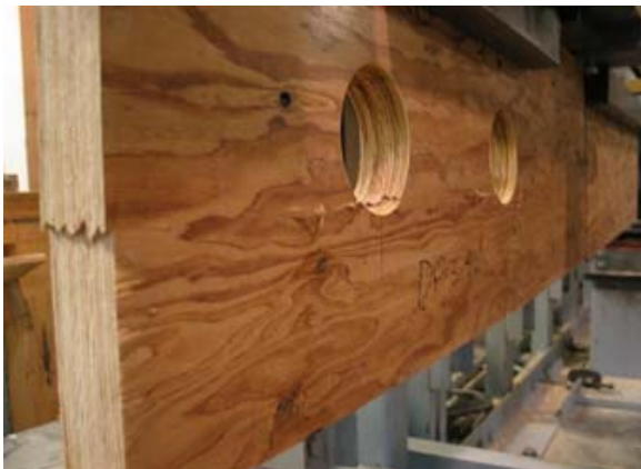
Figure 2. A shear failure mode of a 406-mm (16-inch) deep LVL specimen with two 135-mm (5-1/3-inch) diameter holes at the neutral axis
