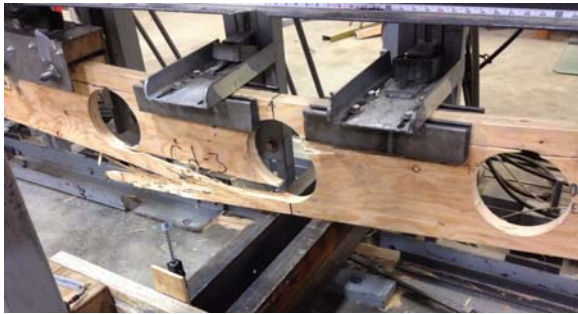
Figure 3. A bending failure mode of a 302-mm (11-7/8-inch) deep LVL specimen with three 203-mm (8-inch) diameter holes at the neutral axis
