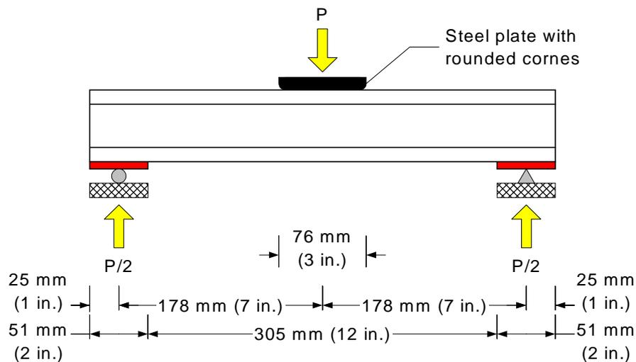
Figure 9. Test setup for edgewise QA shear tests.
