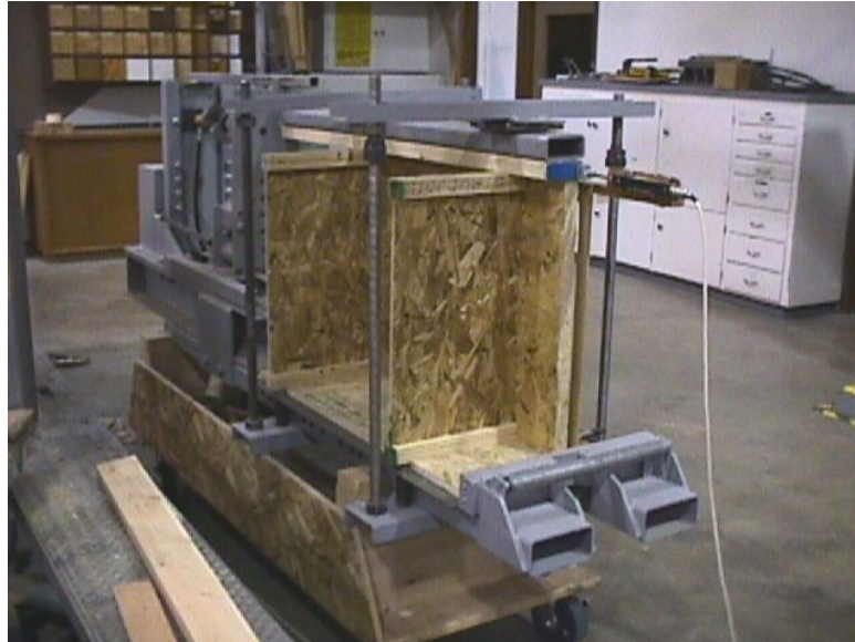
Figure 1. Test setup for horizontal load transfer capacity
