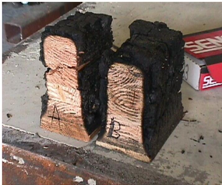
Figure 3. The resulting cross-sections after the fire
