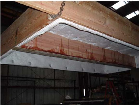
Figure 4. A test beam being installed in the furnace
