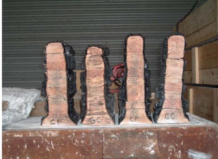
Figure 6. Residual cross sections of tested beams
