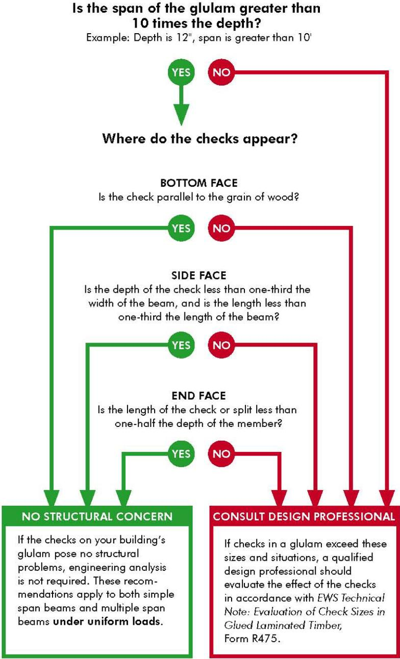
Figure 9. Guidelines for evaluating glulam checks
