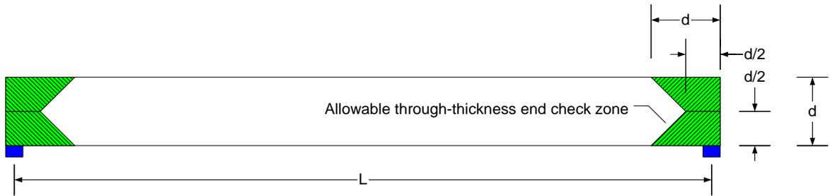
Figure 3. “Green zone” for end checks or splits
