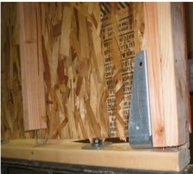
Figure 4. A combination of nail withdrawal, panel edge tear-out, and bottom plate failure from biaxial (combined shear and uplift) tests
