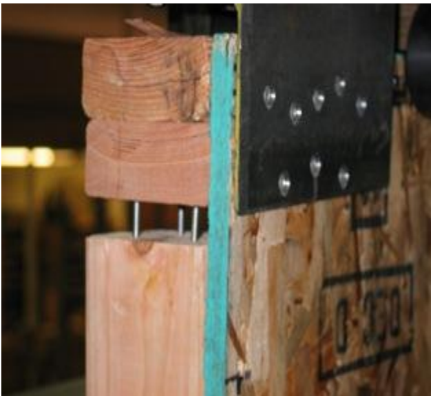
Figure 3. Nail withdrawal from bottom and top plates, and panel edge tear-out from uniaxial (uplift-only) tests
