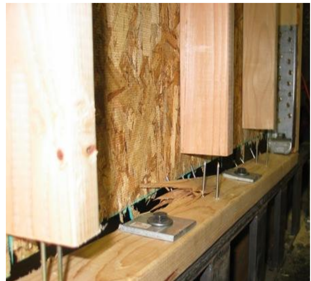
Figure 4. A combination of nail withdrawal, panel edge tear-out, and bottom plate failure from biaxial (combined shear and uplift) tests
