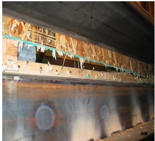
Figure 3. Nail withdrawal from bottom and top plates, and panel edge tear-out from uniaxial (uplift-only) tests
