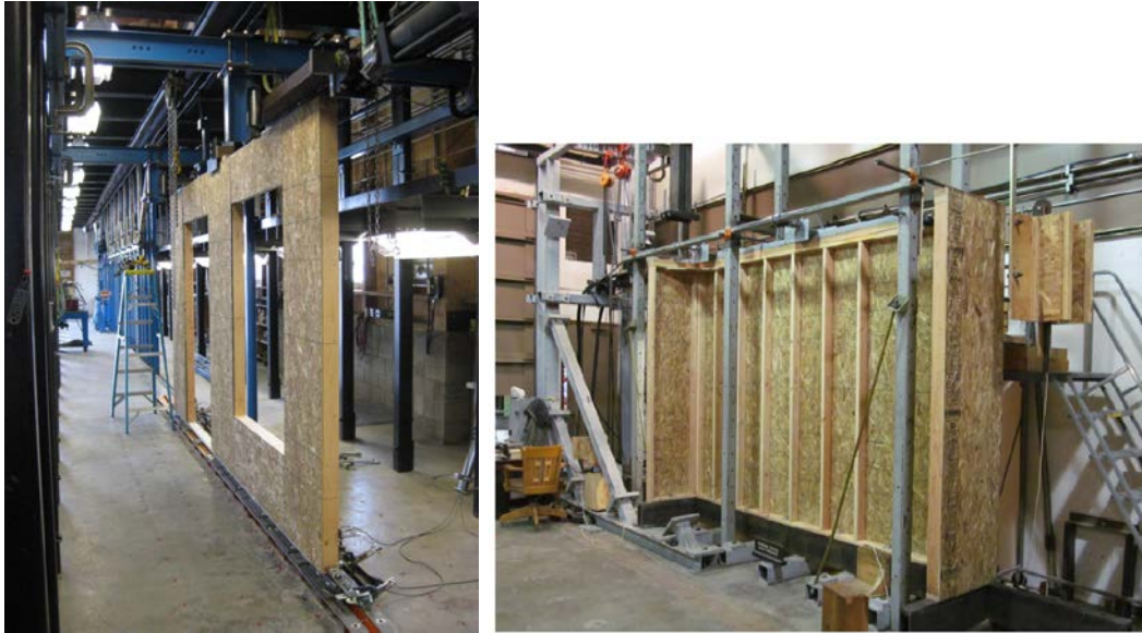
Figure 1: Example Wall Type 7 specimen at Laboratory A (left) and Example Wall Type 2 – corner return specimen at Laboratory B (right)
