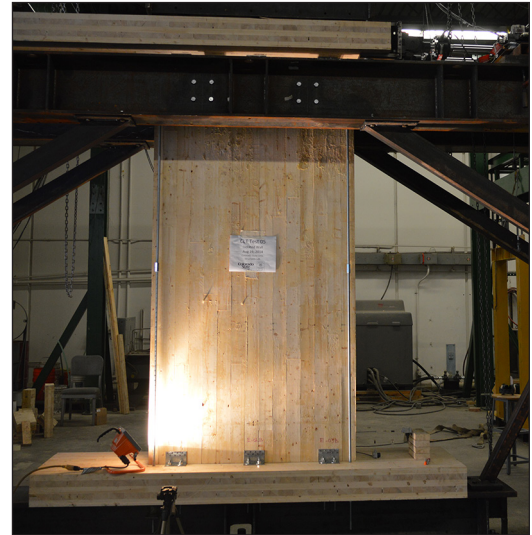
Figure 1. CLT shear wall testing with horizontal actuator in displacement control applying shear load and vertical actuator in load control applying gravity.
