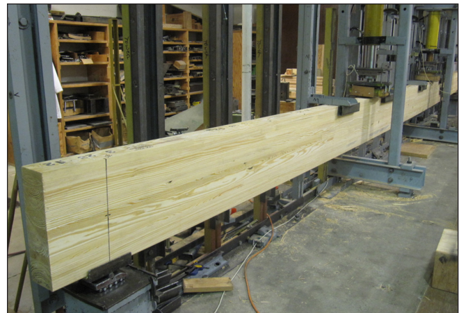
Measuring the bending strength of a glulam beam.
