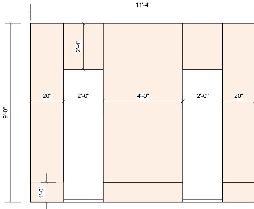
**Figure 8. Series 1B: Panel Placement.**
