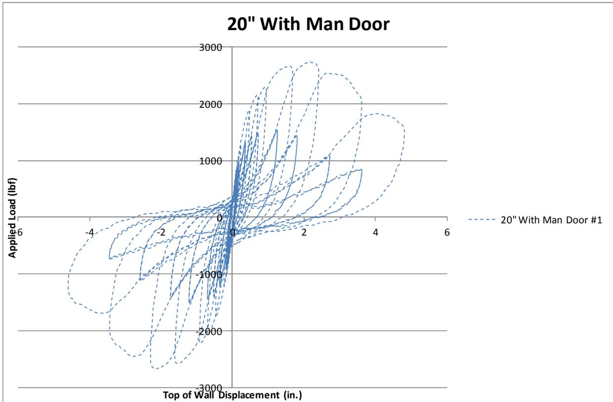
**Plot 10. 20" Element with Man-Door Test Number 1 (1B-1)**
