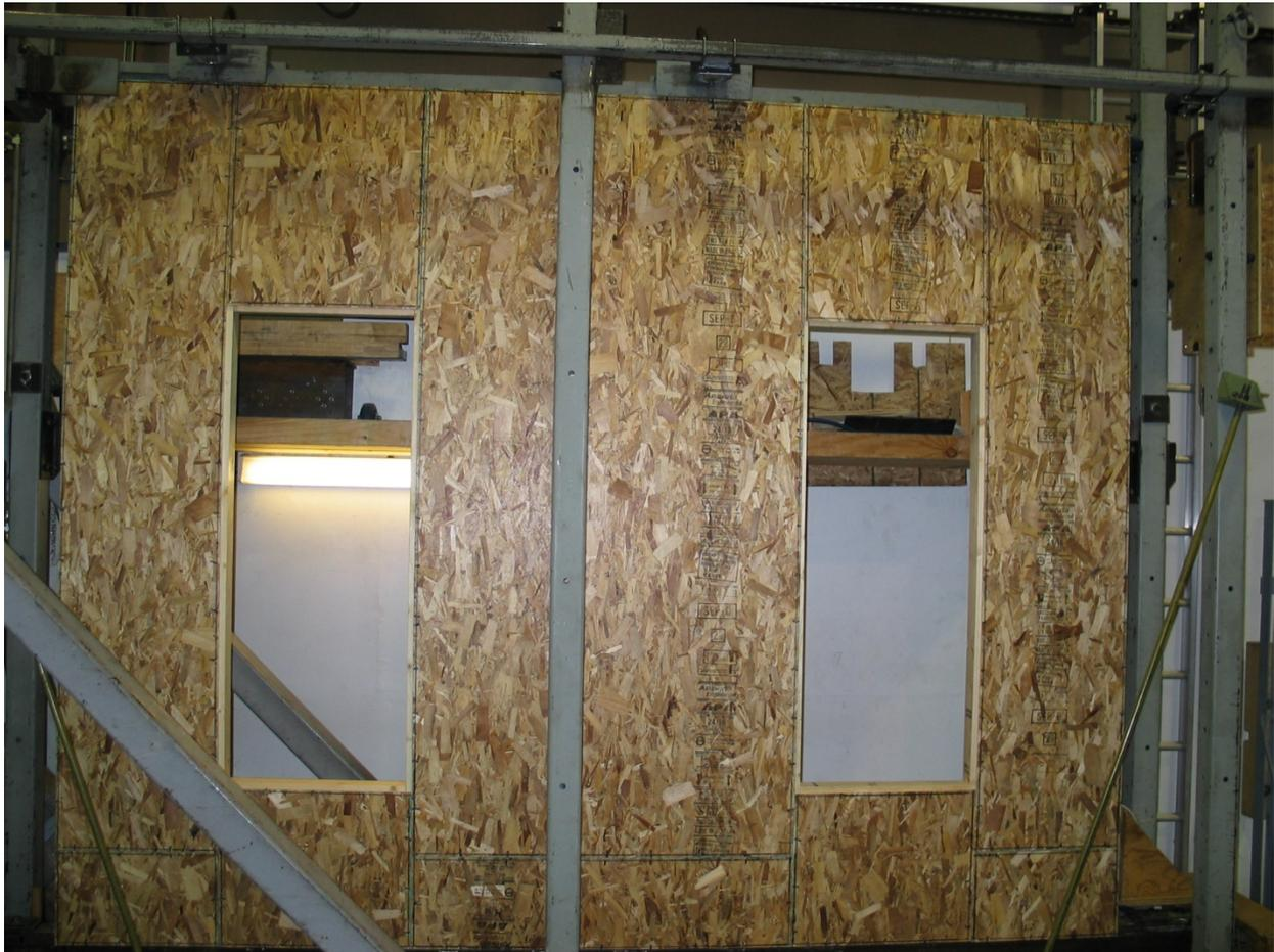
**Figure 7. Cyclic Load Test Machine with Test 2A Wall
