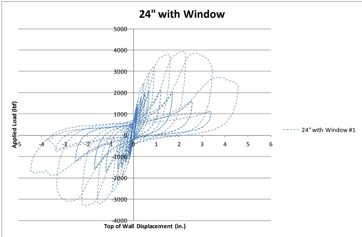
**Plot 7. 24" Element with Window Test Number 1 (2A-1)**
