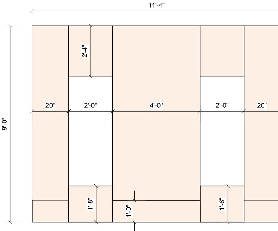
**Figure 9. Series 2B: Panel Placement.**
