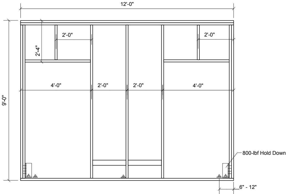
**Figure 10. Control: Framing.**
