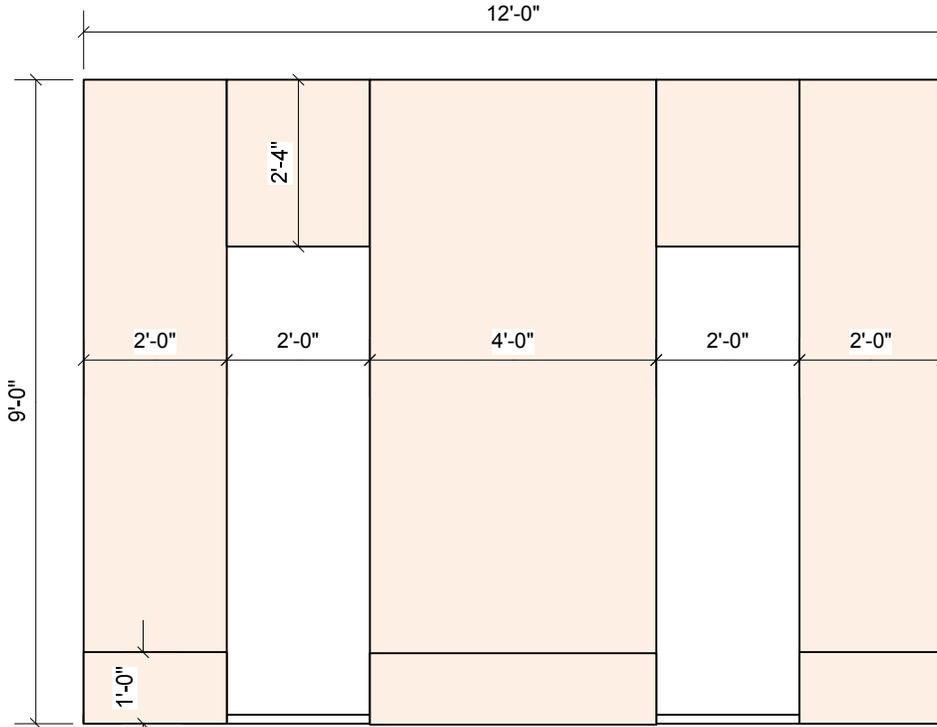
**Figure 4. Series 1A: Panel Placement.**
