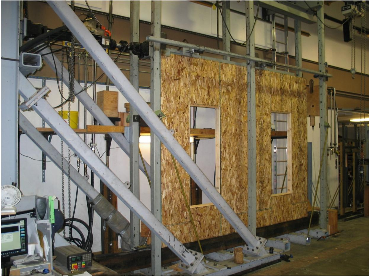
**Figure 1. Test Frame with Test Wall in Place.**
