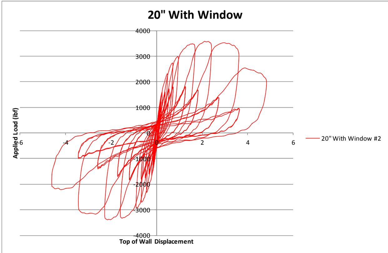
**Plot 14. 20" Element with Window Test Number 2 (2B-2)**
