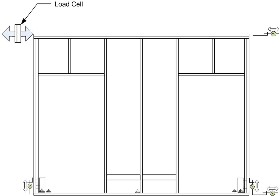
**Figure 15. Instrumentation (Typical).**
