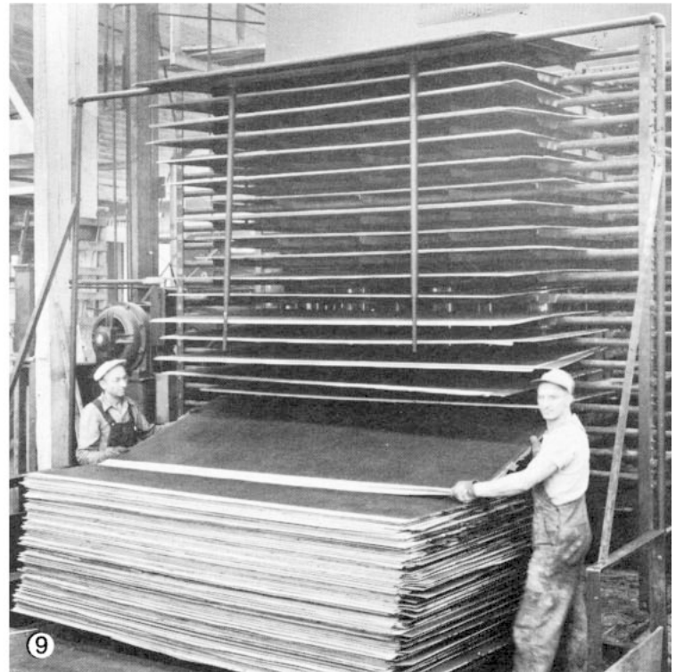
Air view of Buffelen plant in the early 40's (7) shows main plant complex upper center with plywood plant at left. Log pond (8) showing fir and Philippine mahogany logs. Inderon, the first Medium Density Overlaid plywood, coming out of 20-opening hot press (9). Jacques Willis (10) was the originator of Inderon. Henry Mertz (11) led in the modernization of Buffelen plant in the middle 30's. Art Peterson (12) took over as Sales Manager in 1936 when Mertz became General Superintendent.
