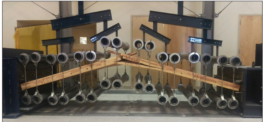
Load tree testing of CLT panels at Tyndall Air Force Base.
