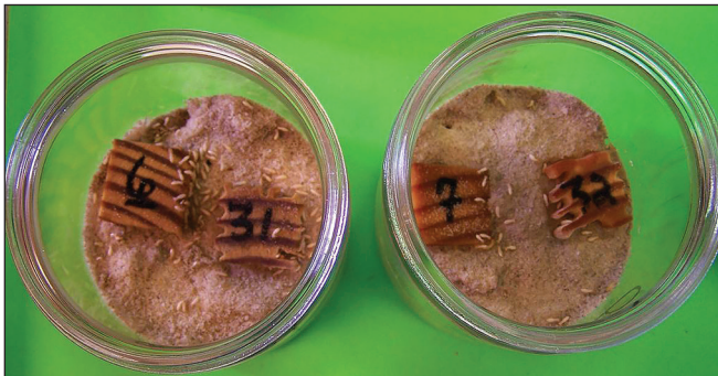
Figure 2—Standard termite feeding test, showing undamaged, protected (samples 6 and 7) and attacked control wood (samples 31 and 32) with termites over the samples. (Courtesy of Linda Sites, Mississippi State University.)
