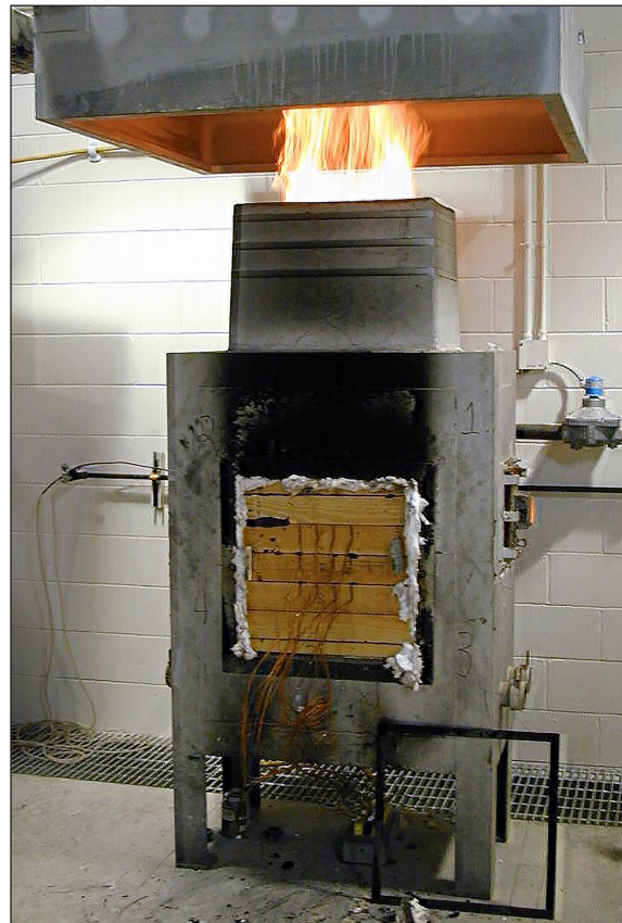
The small vertical furnace at the Forest Products Laboratory.
