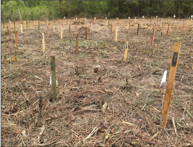
Typical installation of an E7 field stake plot. This field plot is located in Saucier, Mississippi, at the Harrison Experimental Forest. Using this layout, preservative-treated stakes will be installed at two sites and sampled at scheduled intervals. At sampling, bacterial DNA will be extracted and used for next generation sequencing of bacteria present in the wood.
