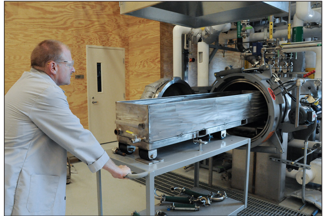
Eighteen-inch-long field stakes will be treated at the FPL wood preservation pilot plant in Madison, Wisconsin, and installed in ground contact at field sites in Wisconsin and Mississippi.
