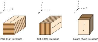
Thickness (t) along Y-axis; Width (w) along X-axis; Length (L) along L-axis [Axes per Figure 1 ASTM D5456]
