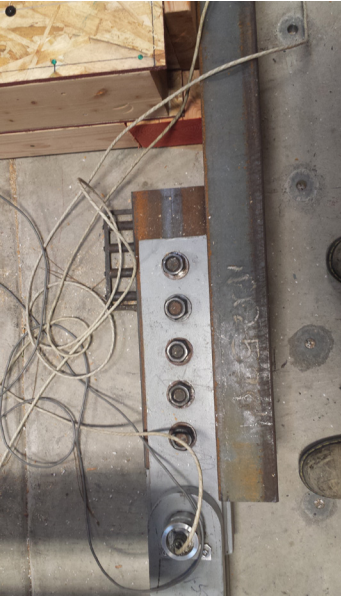
Figure 6. Reaction channel attachment to load cell.
