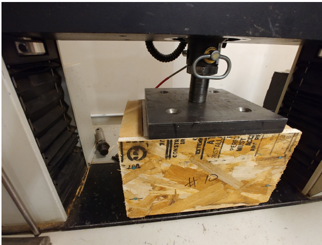
Figure 12. An 8d cooler nail specimen in the test machine.
