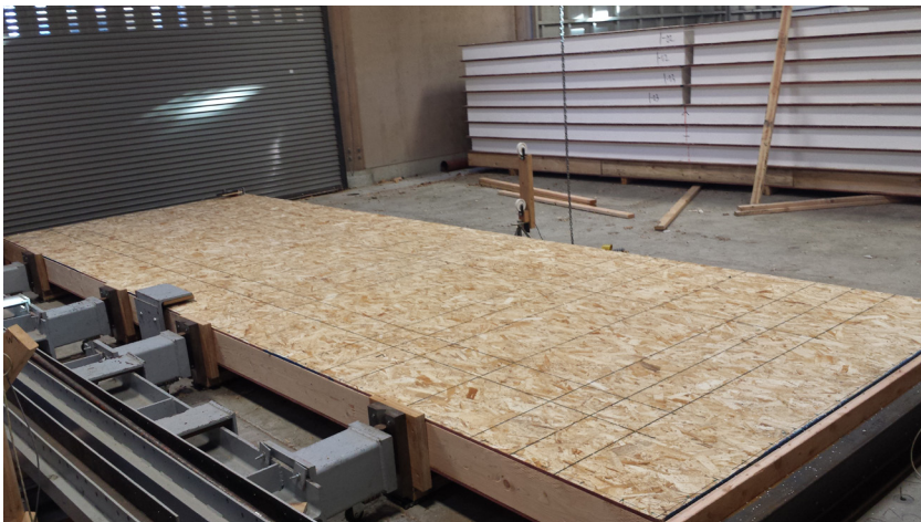
Figure 4. Test setup for a Part A SIP diaphragm (before testing).
