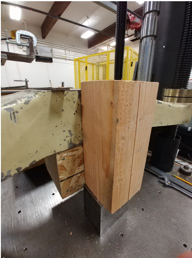
Figure 13. A SIP screw test specimen in the test machine.
