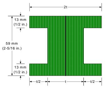
Figure 8. Specimen dimension for small-scale QA shear tests (t = LVL thickness)
