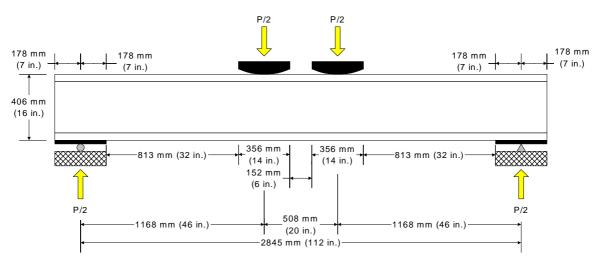
Figure 4. Test setup for LVL edgewise shear tests
