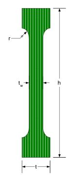
Figure 2. The I-shaped specimen used by Lam and Craig [4] (t = LVL thickness)
