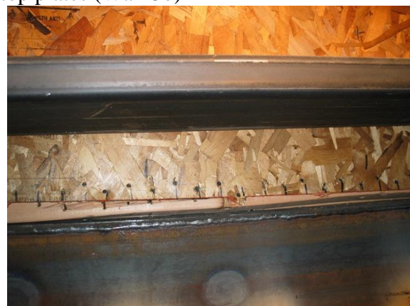
Figure 4. Typical failure mode from combined shear and uplift tests (Wall A5)
