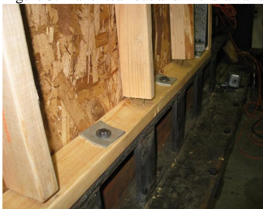
Figure 4. Typical failure mode from combined shear and uplift tests (Wall A5)
