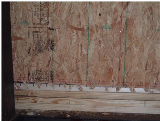
Figure 3. Panel tear-out and withdrawal of top plates (Wall 3b)
