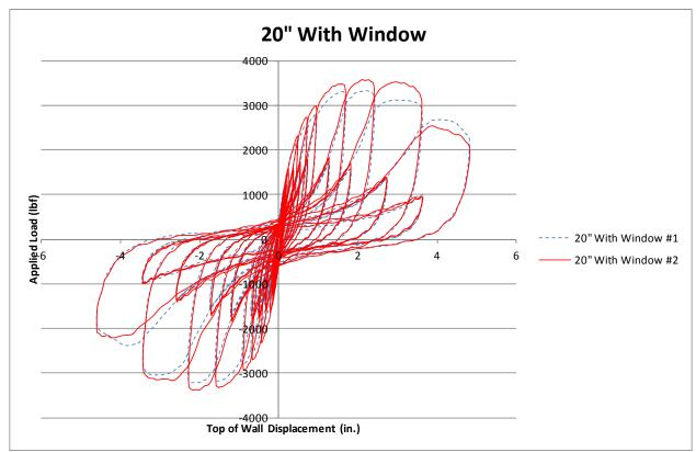
Plot 15. 20" Element with Window Test Numbers 1 & 2 (2B-1 & 2B-2)
