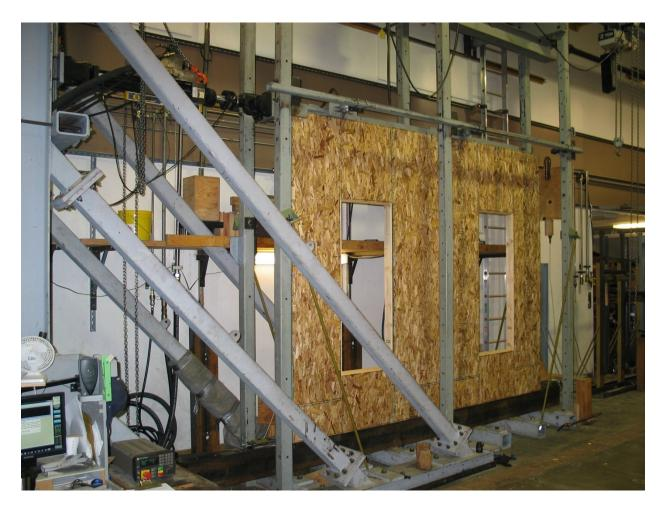
Figure 1. Test Frame with Test Wall in Place.
