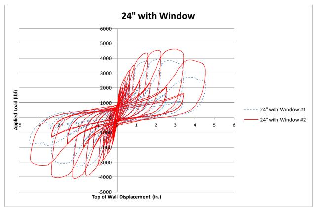
Plot 9. 24" Element with Window Test Numbers 1 & 2 (2A-1 & 2A-2)
