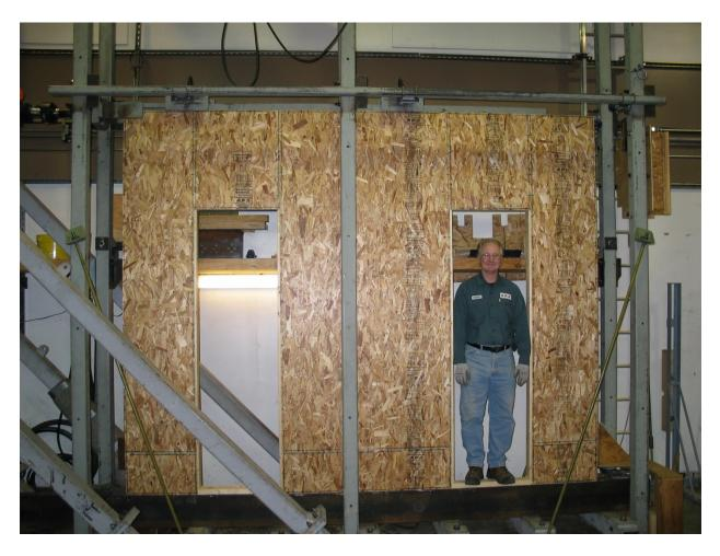
Figure 5. Cyclic Load Test Machine with Test 1A (Test 1B Similar) Wall in Place.
