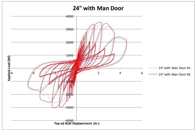
Plot 6. 24" Element with Man-Door Test Numbers 1 & 2 (1A-1 & 1A-2)
