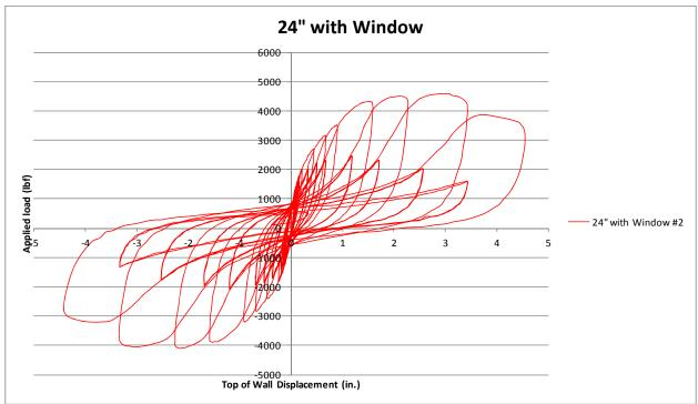
Plot 8. 24" Element with Window Test Number 2 (2A-2)
