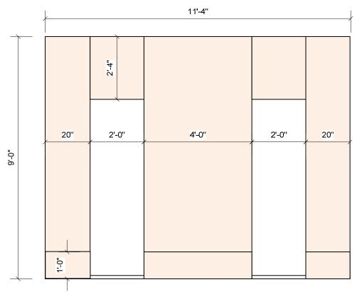
Figure 8. Series 1B: Panel Placement.
