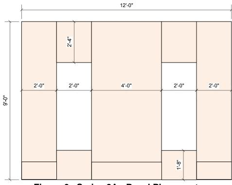
Figure 6. Series 2A: Panel Placement.
