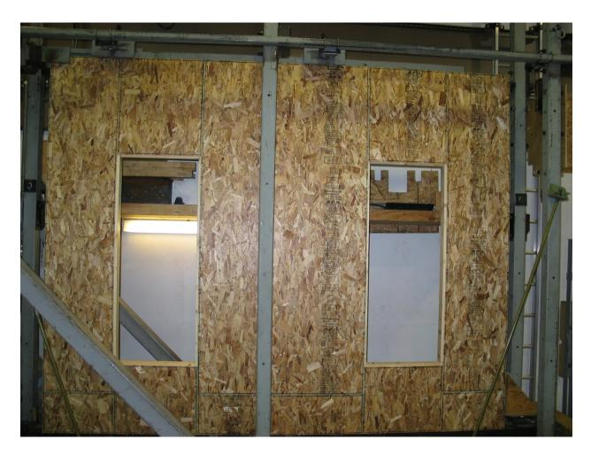
Figure 7. Cyclic Load Test Machine with Test 2A Wall (Test 2B Similar) in Place.
