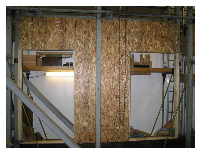
Figure 3. Cyclic Load Test Machine with Test C-1 (Control) Wall in Place.
