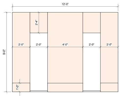
Figure 4. Series 1A: Panel Placement.
