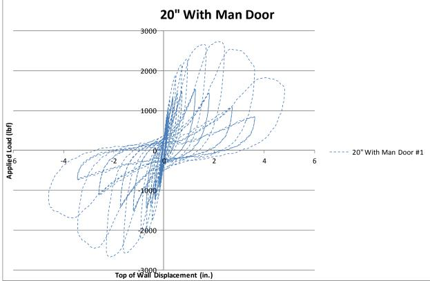
Plot 10. 20" Element with Man-Door Test Number 1 (1B-1)
