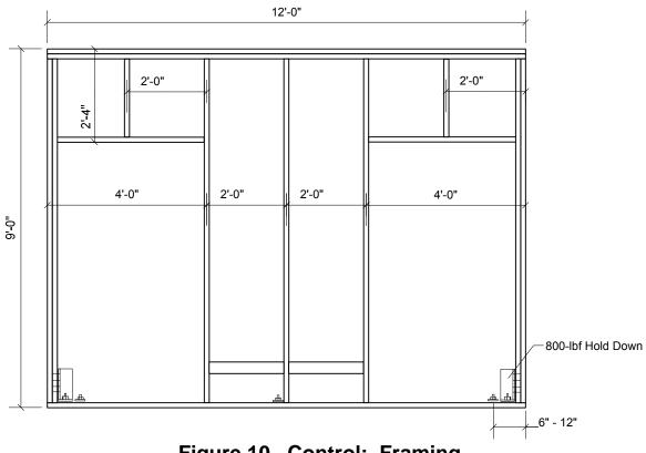
Figure 10. Control: Framing.
