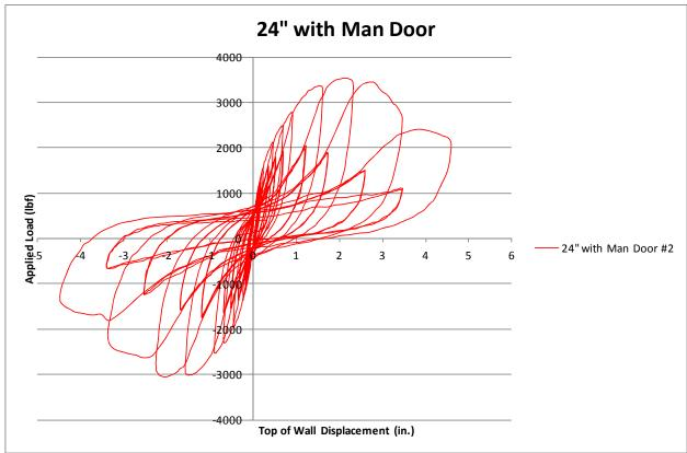
Plot 5. 24" Element with Man-Door Test Number 2 (1A-2)
