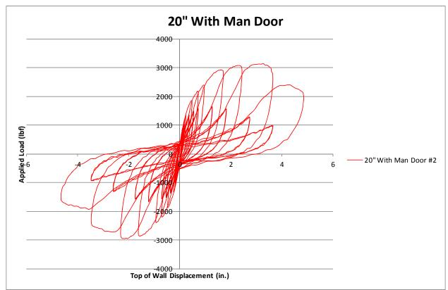
Plot 11. 20" Element with Man-Door Test Number 2 (1B-2)
