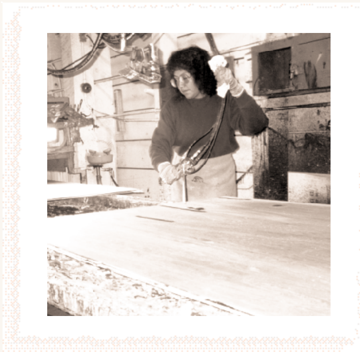
Kathy McWilliams, K Ply shareholder-owner, works on the cureline putting epoxy in drilled splits and knotholes.
