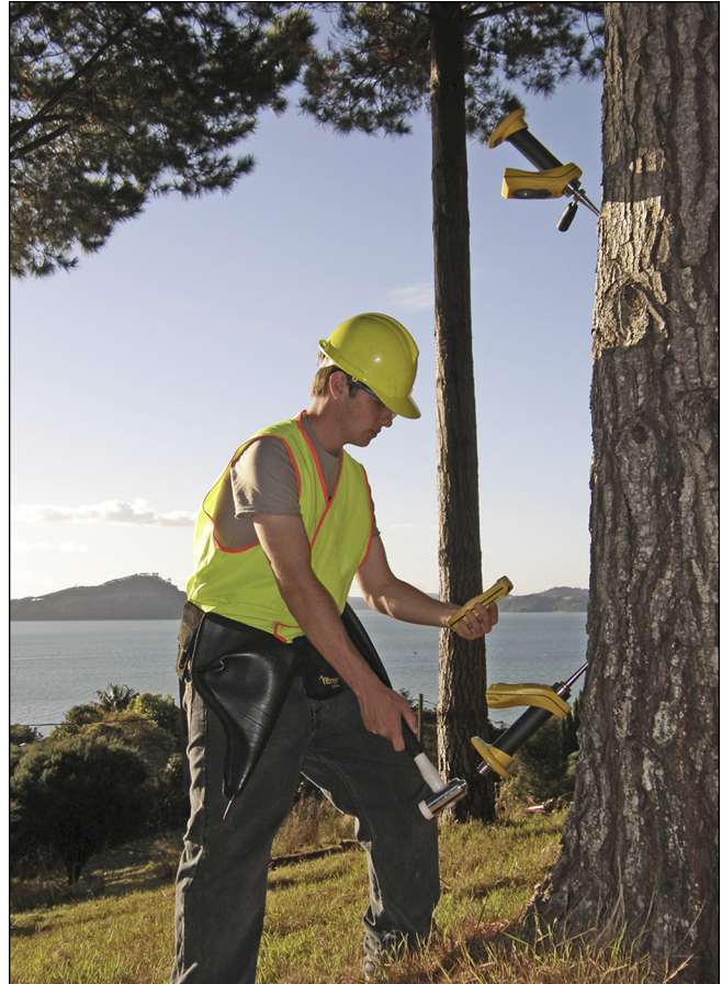
Standing timber being evaluated with a nondestructive testing tool that utilizes ultrasound, lasers, and vibrational characteristics.
