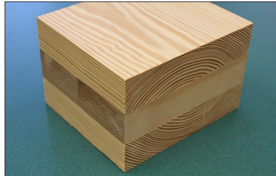
Cross-laminated timber made from mixed species (sugar maple and southern pine).
