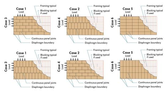
Figure 1. Diaphragm configurations
